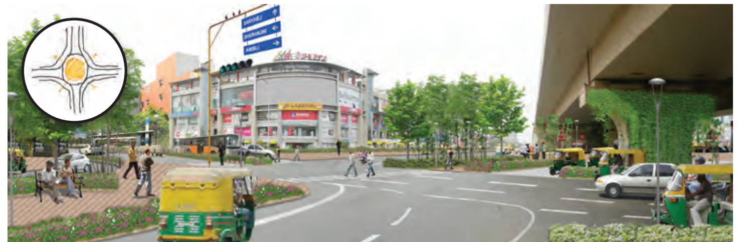
Central Plaza The central plaza concept adds clear overhead traffic signals, signage, and a large landscaped island. The concept removes billboards and overhead cables to streamline sight lines.
